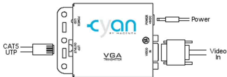
Figure 3-1. Connections on the Cyan VGA Video Extender Transmitter
