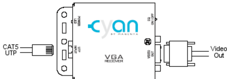
Figure 3-2. Connections on the Cyan VGA Video Extender Receiver
